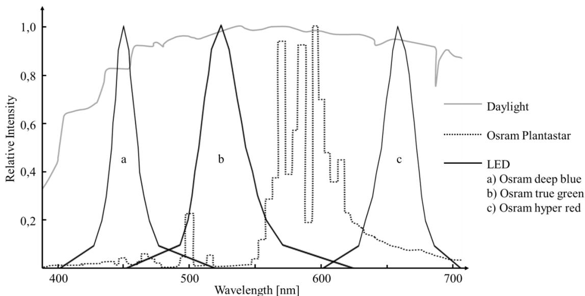
Fig. 1. Relative spectral distribution of radiation of the used light sources (edited; Nilsen, 1971; Osram, 2009; Osram, 2010; Osram, 2011)
